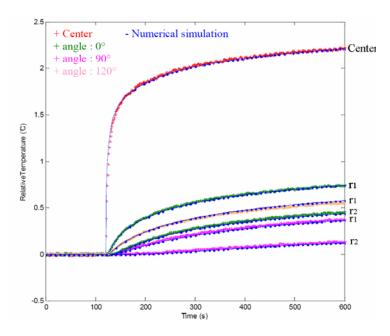
Fig. 5 Heating configuration ①: Experimental and numerical temperature rises for a unidirectional composite sample.
