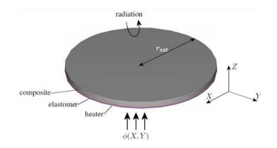
Fig. 3 Finite element geometry scheme containing heater, elastomer and composite fields.
