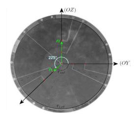
Fig. 2 Upper face of the heater composed of two heating tracks.
